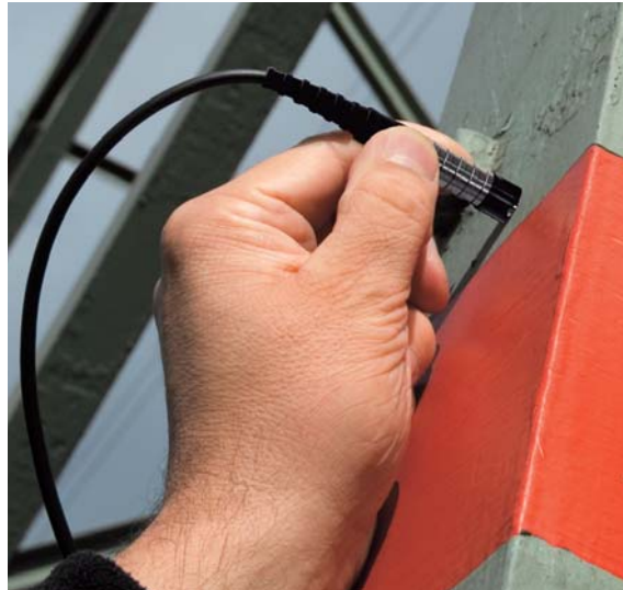
Measuring of duplex coatings with the probe FDX13H
