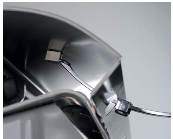
Auto body in section to show how the probe measures the EPD coating within the auto body
