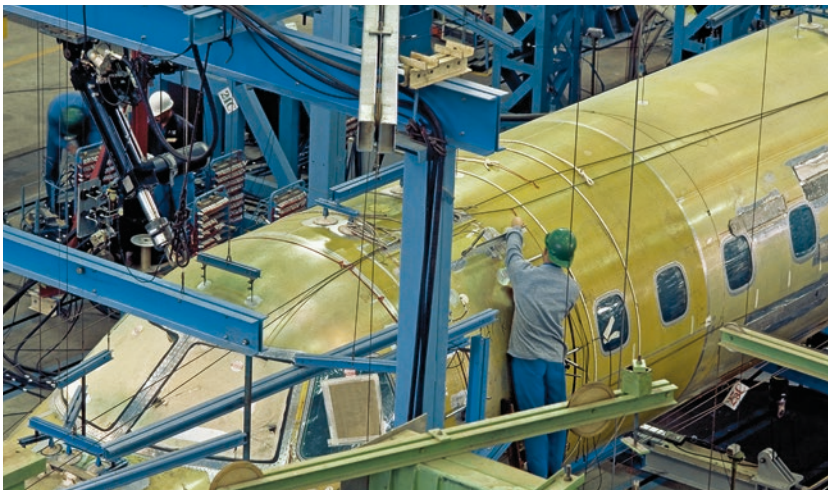
Measuring the electrical conductivity is an important element of quality assurance in the manufacture, maintenance and repair of aircraft
