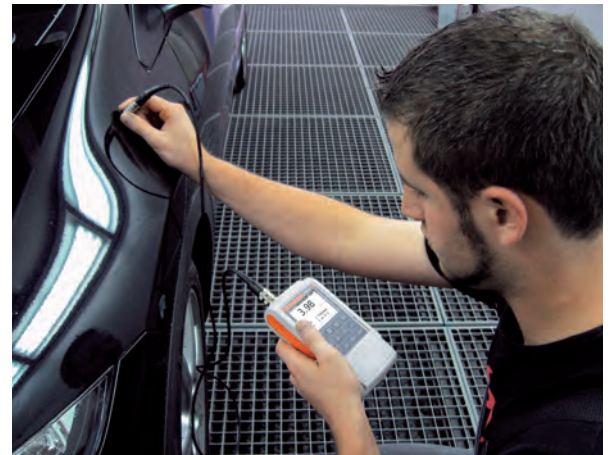
Paint coating thickness measurement using the dual probe FD13H
