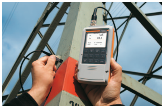
DUALSCOPE® FMP40 using the duplex probe FDX13H
