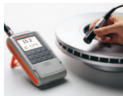
DELTA SCOPE® FMP30 using dual-tip probe V7FKB4
