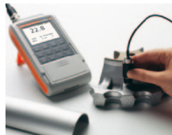
ISOSCOPE® FMP30 using probe FTA3.3H
