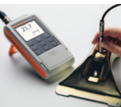
DELTA SCOPE® FMP10 using the probe FGAB1.3
