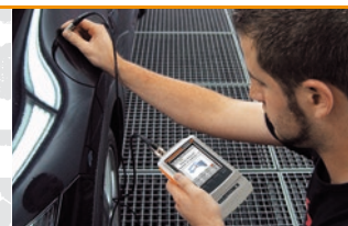
Measurement of auto body paint thickness using the Dual Probe FD13H
