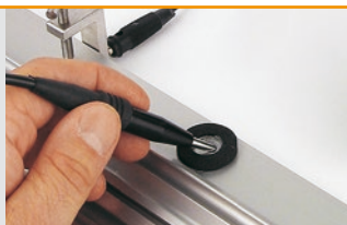
ANOTEST® YMP30-S: Testing the seal of anodized coatings
