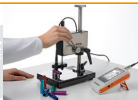
Measurement with support stand on curved anodized parts
