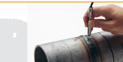
FERITSCOPE® FMP30: Ferrite content measurement on weld seams
