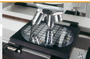
Wafer: Hardness determination on the gold coating
