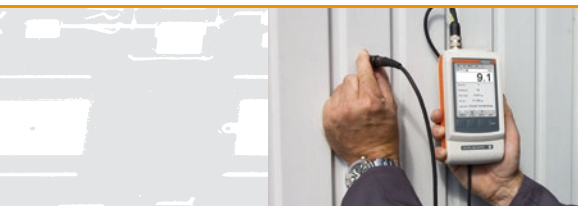
Measuring paint coating on steel
